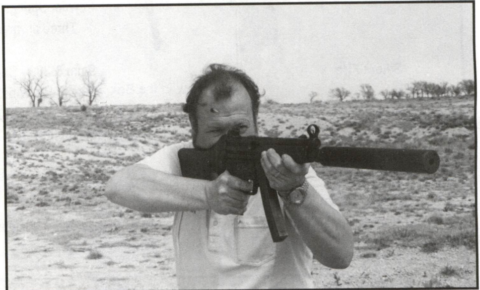
The AP-9 suppressor from Blaylock's Gun Works is a muzzle attachment suppressor which allows 9mm ammo to be suppressed but still used to its highest velocity potential.
